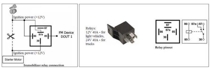
This case fully blocks the ignition while GSM signal jamming is active.
