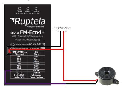
In this case, the driver will be informed by the buzzer that the GSM signal is being jammed.
